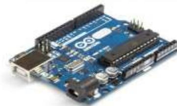
Gambar 1. Papan Arduino Uno R3
